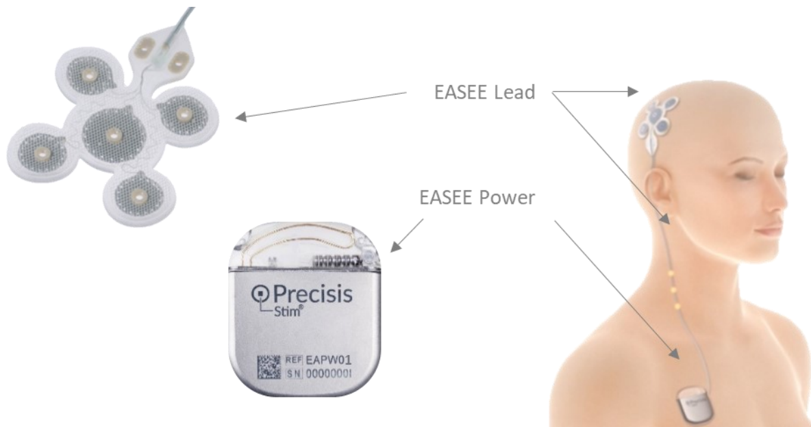
Figure 2 Overview of the Implantable Components of the EASEE System
